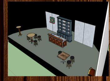
From 'Sketchup' the model is then imported into a lighting software programme called 'Capture' where the lighting positions and techniques can be applied with renderings to produce an image of a certain scene or moment in the play.
